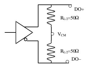
Figure 19. DC Output Reference System Load
