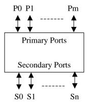
Figure 16. External Model of a Switch
