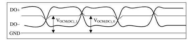
Figure 22.  $V_{OCM(DC)}$
