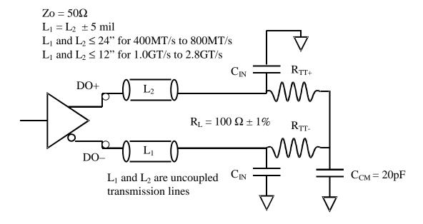
**Figure 25.** AC Reference System Load (See Table 124 for C<sub>IN</sub>, R<sub>TT+</sub> and R<sub>TT</sub>)
