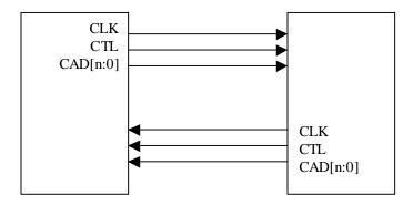
Figure 1. HyperTransport<sup>TM</sup> I/O Link
