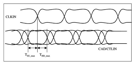
Figure 34.  $T_{SU}$  and  $T_{HD}$
