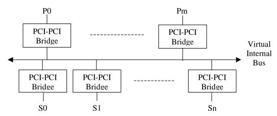
Figure 17. Logical Model of a Switch
